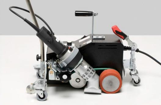
The automatic welding machine FORSTHOFF-P2 is the innovative successor of the successful FORSTHOFF-P models and an efficient and manoeuvrable device for welding truck tarpaulins, tents, awning materials and advertising banners. It produces optionally 40 ,30 ,20 and 45 mm wide overlap welds and may also be converted for welding in welting ropes.
